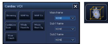
CardioLine+, Cardiac Plane Positioning Support Function, automatically detects anatomic landmarks for accurate and reproducible positioning of the standard views recommended by SCMR.<sup>2</sup> The software uses a set of 3D images, acquired through the chest in a single breath hold, to determine the anatomy and orientation of the heart, automatically aligning for 14 different anatomic views plus one straight axial of the heart.
